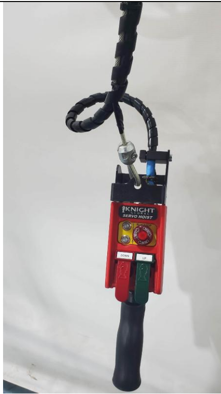
Figure 2-10 Pendant with dual analog levers P/N# KCA1214
