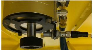
Brake is disengaged and 462PRX is OFF
