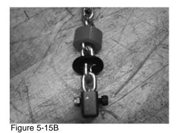
16. Install chain stop, which was removed in step 15, on new chain and place chain stop end into
