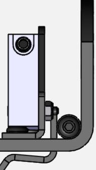
4-pin Micro-Single Pole Limit Switch with 1-N/O (Normally/Open) and 1-N/C (Normally/Closed) contacts.
