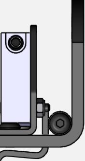
Trigger 4-pin Micro-Single Pole Limit Switch with 1-N/O (Normally/Open) and 1-N/C (Normally/Closed) contacts
