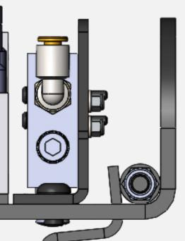
Trigger 4-way valve used for sending pilot signals
