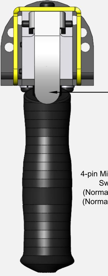
4-pin Micro-Single Pole Limit Switch with 1-N/O(Normally/Open) and 1-N/C(Normally/Closed) contacts.
