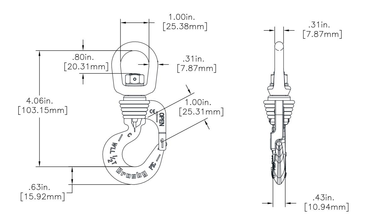
HOOK w/CLOSED SWIVEL BAIL and SELF CLOSING GATE (X) REQ'D  $\sim$  CROSBY/BULLARD BLC SERIES 1050210 w/LIF-LOK GATE
