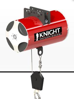
Air Balancers are used in applications where a "float" condition is beneficial. Float allows for the hands-free final positioning of an object. The up/down speed of a air balancer is quicker when compared to a hoist and allows for a "feathering" operation when locating the load. The pendant controls are ergonomically designed incorporating color coded thumb levers. Reeving a air balancer increases the mechanical advantage of the product.
