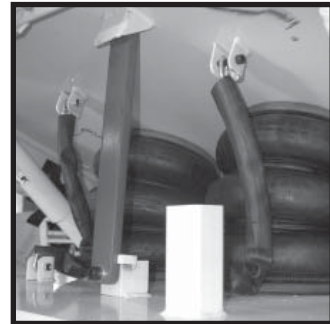
Tilt Maintenance Bar (Engaged Position)
