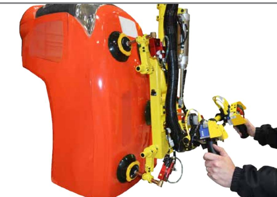
Knight designed a servo and pneumatic operated Vacuum Style End Effector that is accurately maneuvered by Knight's overhead mounted KSHCA Series Articulating Arm.
